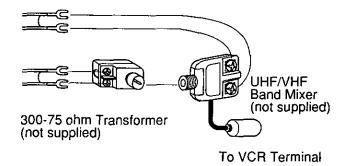
If your TV has both post and plug-type VHF terminals, the post connection is recommended to minimize signal loss.
